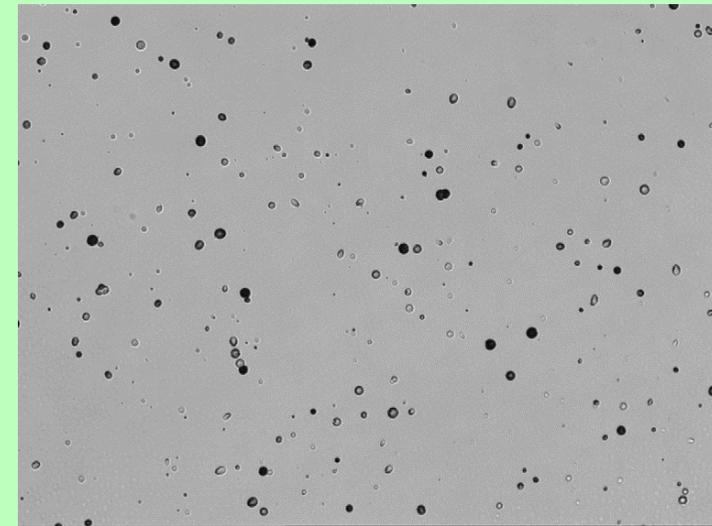
As a result most etch tracks are small and appear circular under the microscope
