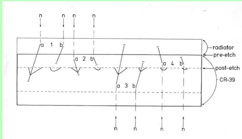
Such recoils can occur either in an overlying radiator or in the plastic itself, leading to a multitude of possible etch track shapes
