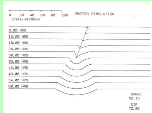
This is illustrated in these simulations of proton etch tracks: upper, 1 MeV; lower, 2 MeV
