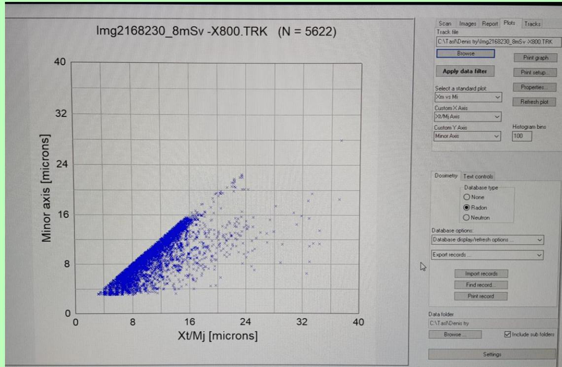
Note that the size envelope is smaller than for  $\alpha$ -particles
