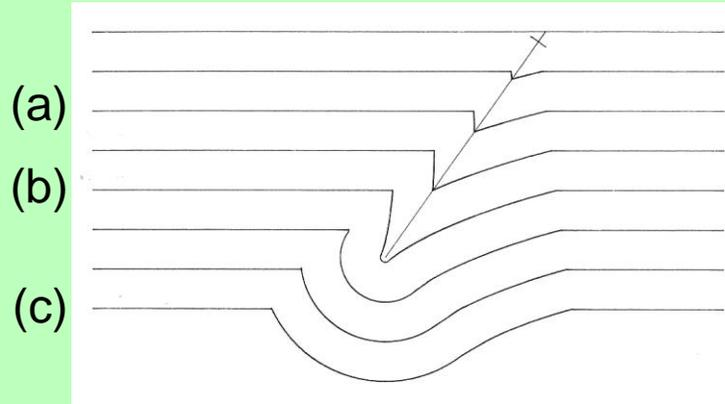
Simulated vertical section profile of the growth of etch pit along the trail of a  $^{218}\text{Po}$   $\alpha$ -particle with range  $40\ \mu\text{m}$  and dip angle  $55^\circ$  in TASTRAK plastic. Etching is at  $98^\circ\text{C}$  in  $6.25\ \text{M NaOH}$ .
