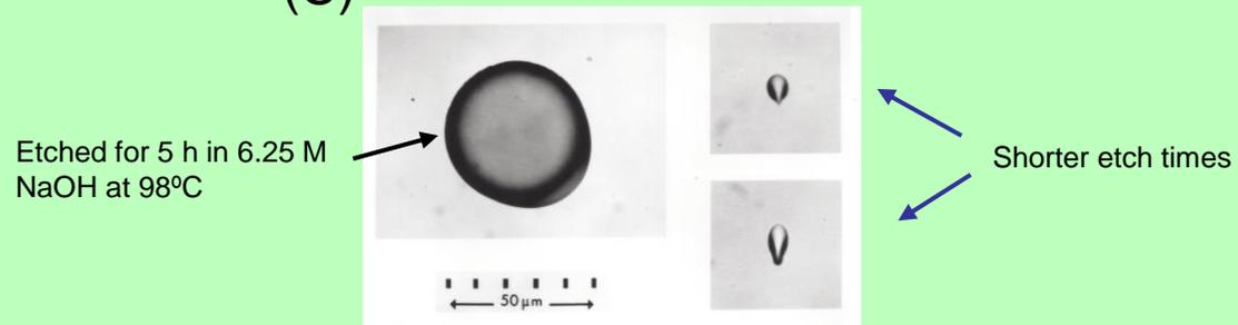
**Note:** there is a minimum level of ionization that will result in a joined-up trail of damage that will then result in preferential etching as described in (B) and (C). For this reason, TASTRAK is a selective detector that does not record tracks of beta-particles or gamma radiation. It will, however, record protons up to several MeV in energy, making it ideal for use in fast neutron dosimetry via recoil protons in the plastic.
