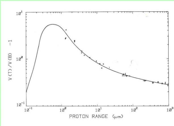
The etch rate ratio  $V(T)/V(B)$  is lower along proton compared with  $\alpha$ -particle tracks
