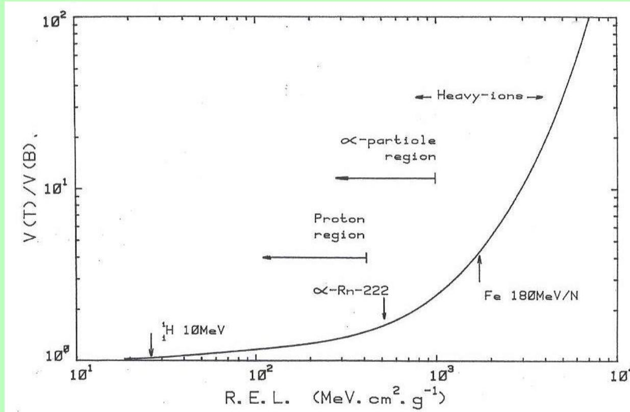
Note that the  $\alpha$ -particle response falls in the central portion of the response curve. In contrast, the proton response merges into the ionisation threshold response. As a result, small changes in the threshold response can alter the response to the spectrum of recoil protons recorded in fast neutron dosimetry.
